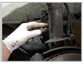
Use a socket wrench or impact gun to remove the 15 mm nut on the front sway bar endlink.
