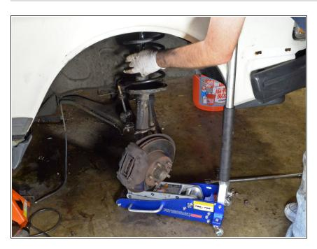
Slowly lower the jack and guide the strut assembly down and out of the car.
