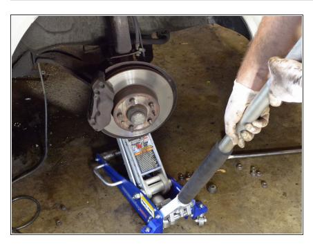
Place a jack underneath the ball joint to support it once you remove the 3 ball joint-to-control arm bolts.
