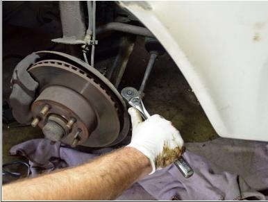
Use a socket wrench or impact gun to remove the 19 mm tie rod end nut.
