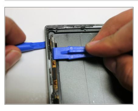
With a plastic opening tool, push out the power button from the left side of the tablet.
