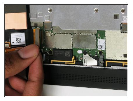
Disconnect the connector from the tablet.
