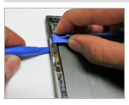
Using a plastic opening tool, push out the volume button from the left side of the tablet.
