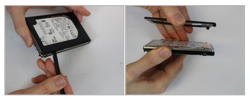
• The top plastic piece is adhered with a weak adhesive. Gently pry it off with a spudger.
