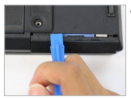
Using a plastic spudger, pry off the plastic cover by pulling it out.
