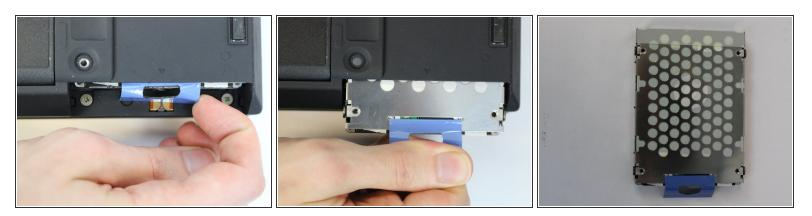
• Utilizing your fingers, untuck the tab and pull to remove the hard drive.
