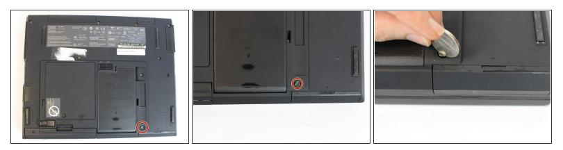
• Using a coin, remove the coin screw by turning counterclockwise.
