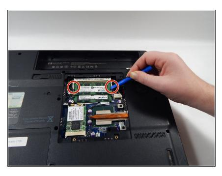
Using the plastic opening tool, open the locks by inserting the tool on the side of the beige locks to release the RAM.
