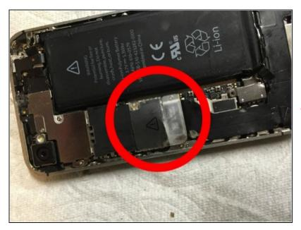
• Locate and pull the Plastic tab to pull out battery. Make sure to pry up outsides of battery on other sides as well.
