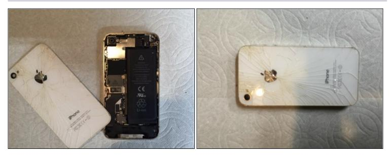
• Push the back panel towards the top edges of the iPhone. Doing this should allow the back to slide off.
