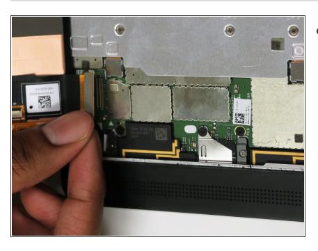
Disconnect the connector from the tablet.
