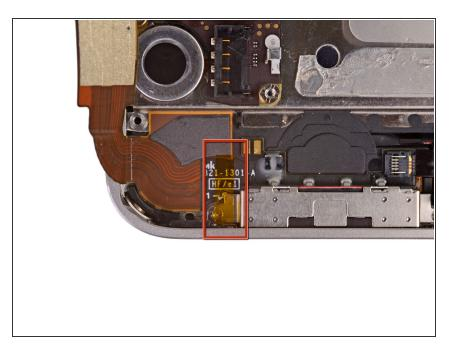
If present, remove the small strip of tape covering one of the dock connector screws.
