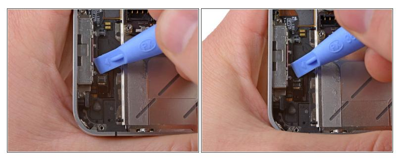
• Use a plastic opening tool to flip up the retaining flap on the home button ribbon cable ZIF socket.
