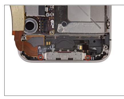
Remove the two 1.3 mm Phillips screws securing the dock connector to the case of the iPhone.
