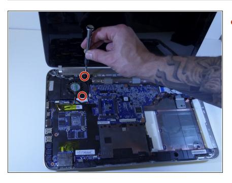
Remove two 5mm screws securing fan, using PH1 screwdriver.
