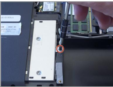
Remove a 3.5 mm screw that is securing DVD player with screwdriver PH1.
