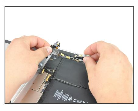
Carefully peel the front camera cable off the bottom ribbon cable attached to the headphone jack. To reassemble your device, follow these instructions in reverse order.
