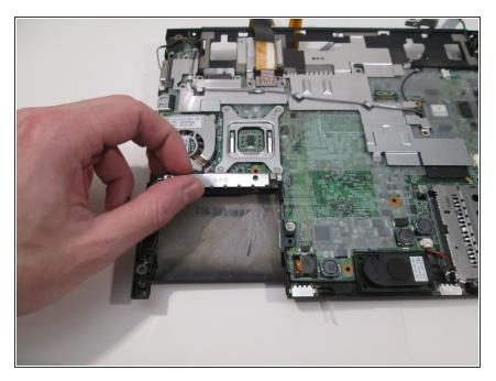
Remove the metal bracket by pulling it up.
