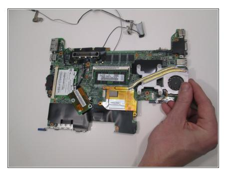
Holding the fan move the whole assembly to the left past the notch holding it in.
