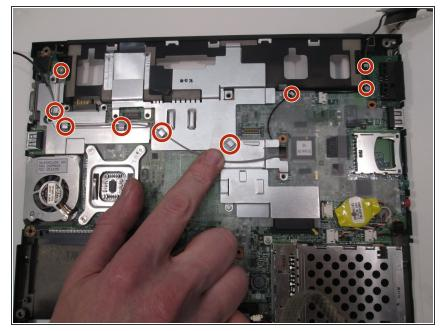
Remove the metal plate covering the motherboard by removing the gray wire from the indicated hooks and pulling the plate up. While you are here remove the other black wire from the indicated hooks as well.
