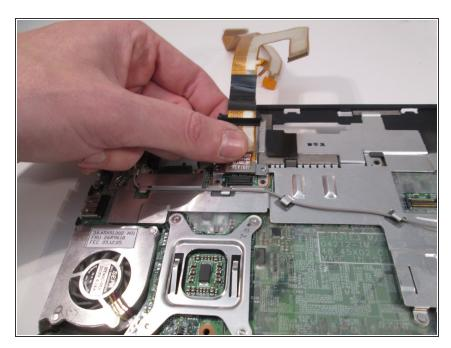
Remove the display connection by pulling it up.
