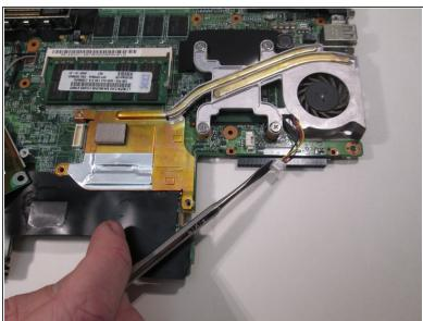
Remove the white tab below the fan by pulling it to the right.
