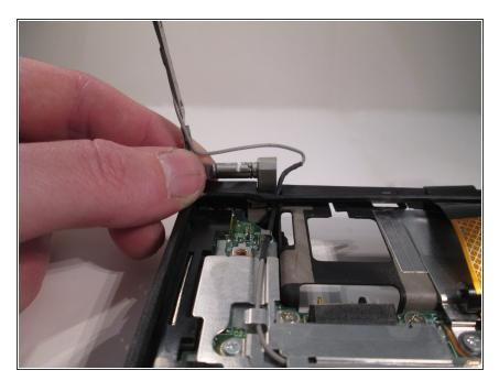
Pull up on the metal hinges to remove the display that is held in on the two sides of the laptop.
