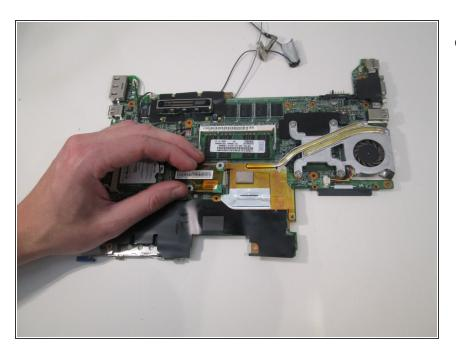
Pull the chip attached to the top of the heat sink and move it to the left.
