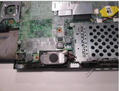
Remove the white tab at the bottom connected to the speaker by sliding it to the right.
