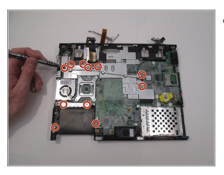
Remove the indicated 4mm screws with a philips head screwdriver.
