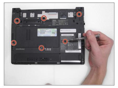
With a Phillips PH000 to remove all six 6 mm screws identified for the keyboard as shown.
