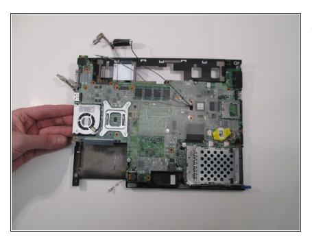
The motherboard can then be removed by pulling it up from the left side.
