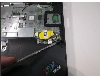
At the bottom right of the laptop remove the black cylinder by lifting it up and out of the depression.
