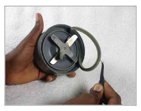
Use tweezers to peel back the rubber gasket that surrounds the inner ring of the lid.
