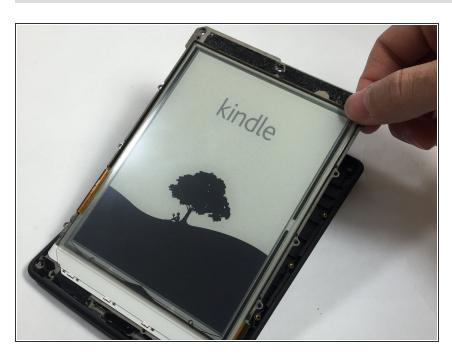
Carefully lift and remove the midframe.
