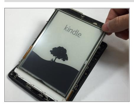
Carefully remove the mid-frame from the back cover.
