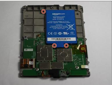
Use a screwdriver to remove the three 3.0 mm Phillips 000 screws that are holding the battery in place as shown.
