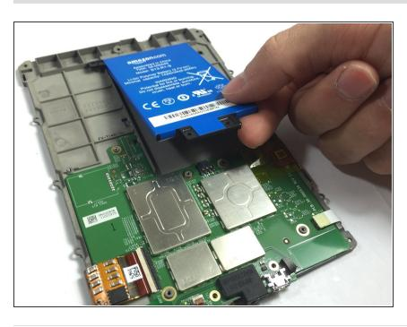
Carefully lift the battery and remove it from the device.
