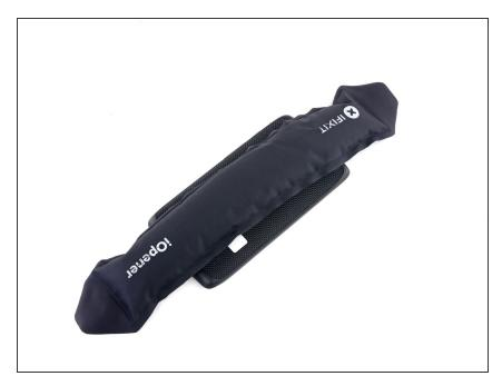
Prepare an iOpener and lay it over the rear case to soften the adhesive on securing the rear case to the phone.
