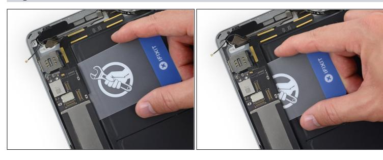
• Insert a plastic card underneath the lower end of the logic board, directly underneath the display connectors and Wi-Fi module.
