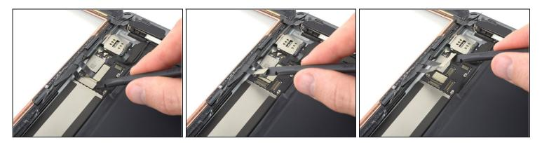
• Use the flat end of a spudger or a fingernail to carefully pop the two digitizer cable connectors straight up from their sockets.
