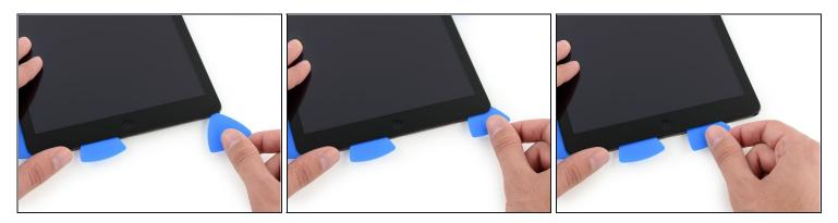
• With the adhesive loosened, you can now insert the pick near the right-hand corner. Slide the pick to the left, and stop just short of the Home button.
