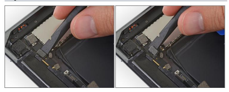
• Use the flat end of a spudger to lift the primary cellular antenna connector from its socket on the logic board.
