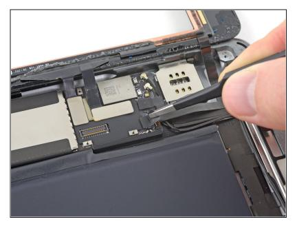
Remove any tape covering the home button ribbon cable connector.
