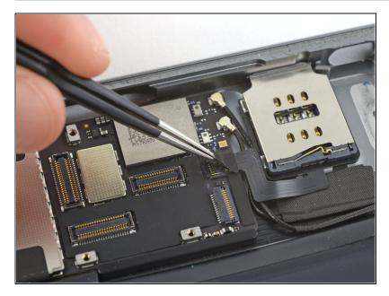
Use tweezers to peel and remove the piece of tape covering the SIM board cable connector on the logic board.
