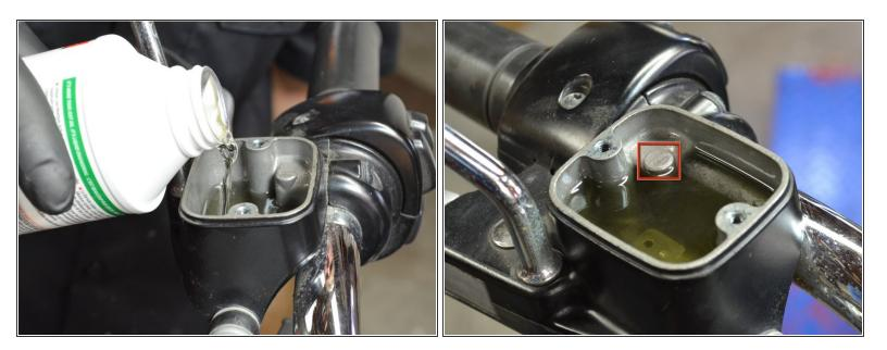
Fill the master brake cylinder one last time with fresh brake fluid until the fluid is level with the metal tab in the rear right corner of the cylinder.
