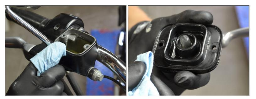
Using a damp rag, wipe down the rim and rubber gasket of the master cylinder and the master cylinder cover.
