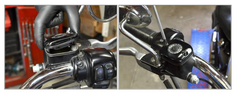
Using a Phillips #2 screwdriver, replace the master cylinder cover and screw it firmly into place.
