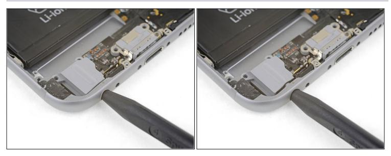
• Insert the point of a spudger into the headphone jack and push to loosen the jack from the rear case.
