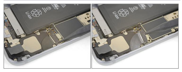
• Use the point of a spudger to lift up and disconnect the Lightning connector ribbon cable from its socket on the logic board.
