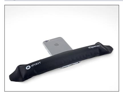
• <u>Heat an iOpener</u> and apply it to the back of the phone near the bottom edge for one minute.
