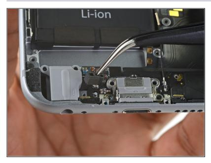
• Remove the plastic microphone bracket.
