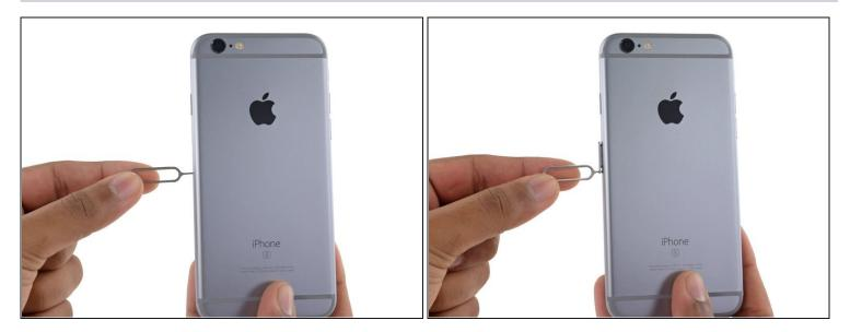
• Insert a SIM card eject tool or a paperclip into the small hole in the SIM card tray.
