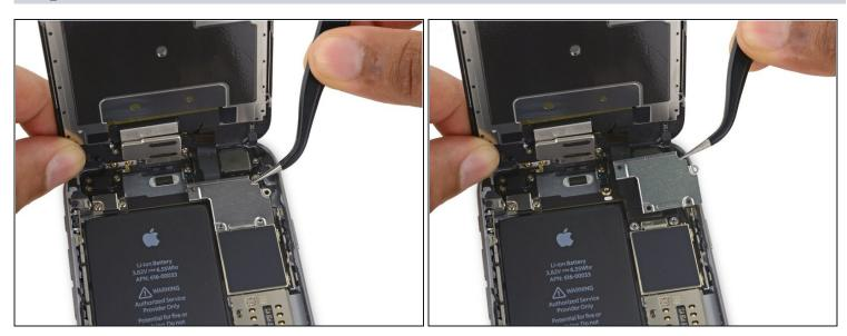
• Remove the display cable bracket.
