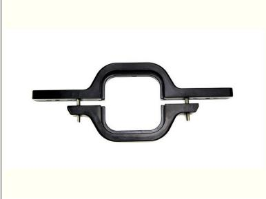
Loosen the screws enough to slightly pull apart the two brackets, then clamp the bracket over your tow hitch with the grooves facing inward and tighten the two screws to secure the tow hitch mounting bracket
