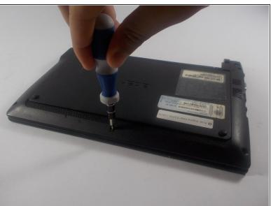
Unscrew seven 1.2 mm Phillips #1 screws from the back of the device
