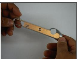
Now with the camera completely disassembled, take the silver trim with the zoom and find the two screws holding the zoom-button assembly.
