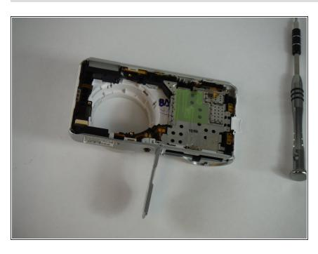
Having completed the previous guides up to this point you should be left with the chassis and internal frame exposed
