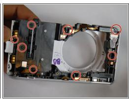
Start by removing nine (4mm, PH00) of the screws which hold the outer silver trim bezels to the main chassis highlighted in red.
