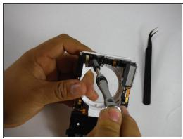
Using the iFIXIT curved nose tweezers, gently remove the ribbon cable for the flash. Doing so will
