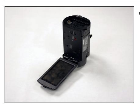
Orient the camera with the battery side facing up.
