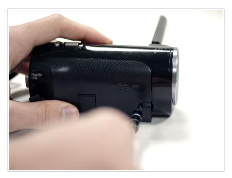
• Turn the camera around to the grip side and remove the 5.5 mm Phillips Head screw using your J00 Phillips Head screwdriver.
