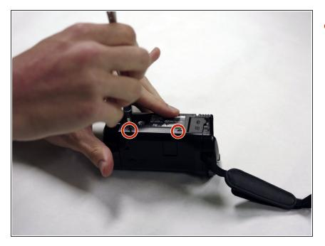
With the bottom of the camera facing up, remove the two 5.5mm Phillips #00 screws.
