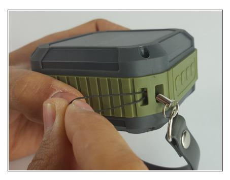
Pull the end of the loop through the device as far as possible.
