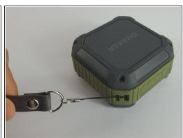
• Feed the end of the strap through the loop. Pull the strap tight until it is secure.
