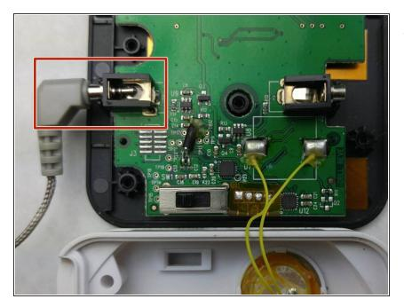
Using a pair of tweezers, bend the probe contacts back in place. The tweezers will touch the probe terminals when inserted.
