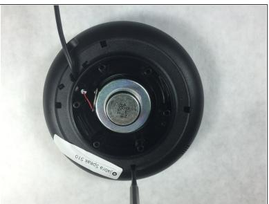
Remove the back plate and the grey foam underneath.
