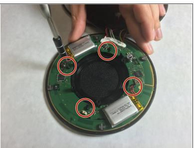
Using the T6 Torx Screwdriver, remove the four (4mm) screws.
