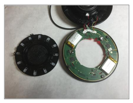
After removing the screws, take out the center covering to free the motherboard by lifting the tabs and pulling it off.
