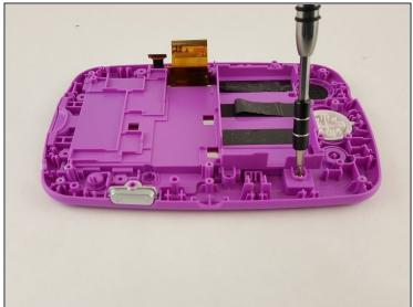
• Unscrew the eight 6.5 mm phillips screws from the plastic casing.
