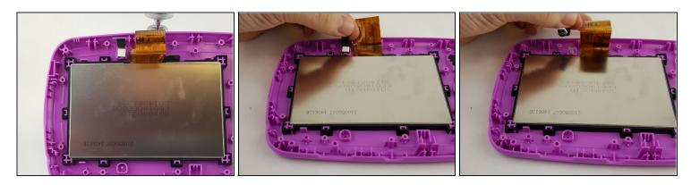
• Remove the front facing camera from the outer case.
