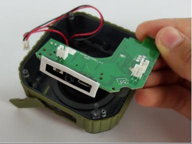
Carefully remove the motherboard with your hand by lifting it from the device.
