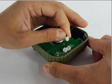
Remove the mic wire by carefully pulling the plug out of the socket.
