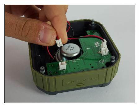
Remove the speaker wire by carefully pulling the plug out of the socket on the motherboard.
