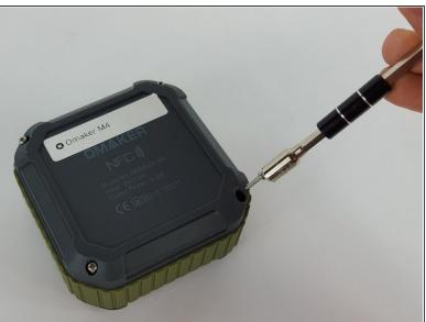
Use a magnet to remove the screws after unscrewing them and place them aside.
