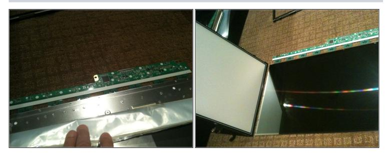
Gently flip the PCB over 180deg so it is off the aluminum back panel.
