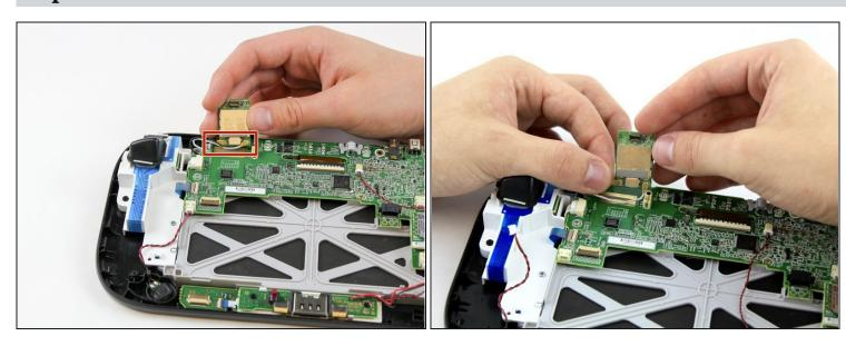
Disconnect the black and white wires off of the back of the WiFi module.
