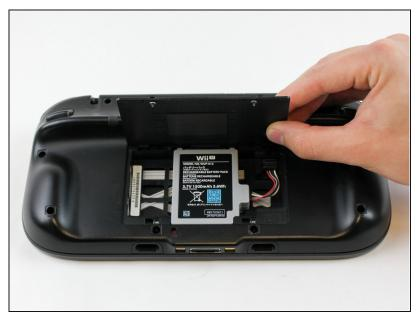
• Lift and remove the battery plate.
