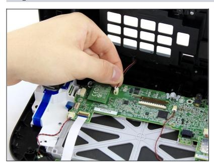
Unplug outer case rumble motor connector from the motherboard with your fingers.
