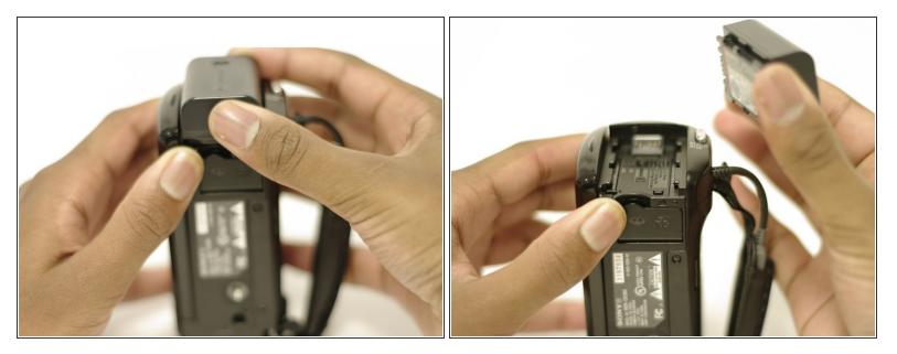
• Using your right index finger and thumb, pull the battery toward you and then away from the camera.
