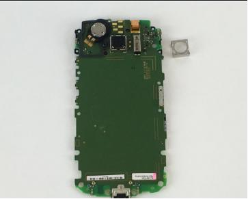
• Using a spudger (ignore the pictured screwdriver), pry up the metal square frame on each side until it comes off.
