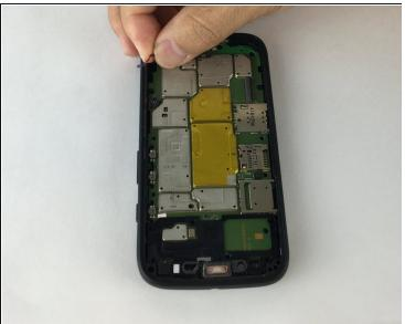
Gently lift up the battery cable connector, it should come out very easy.
