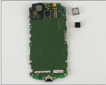
Once the metal square frame is out, use the same tool to pry up the camera by gently pulling on each side until it comes off To reassemble your device, follow these instructions in reverse order.
