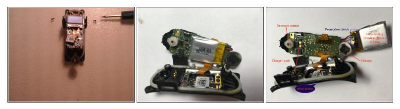
• To access the lipo, remove the two screws above the screen. Pull the circular vibrating motor out and pull out the board.
