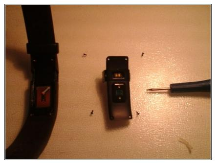
Remove all four T3 Torx screws. Then "pop" out the electronics by pressing in the reset hole and pushing out the side with a pin. Use your thumb and push it up towards the wrist band clip (top in this picture). The unit "slides" up and out.
