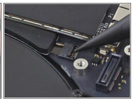
Use the tip of a spudger to flip up the retaining flap on the right fan ribbon cable ZIF socket.
