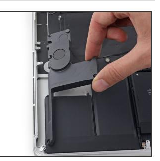
Remove the right speaker by pulling it slightly away from the side of the upper case, and out from under the aluminum tab blocking it in.
