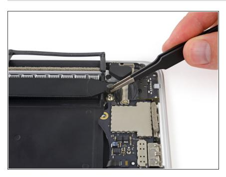
Remove a small rubber cap off the screw at the end of the heat sink.
