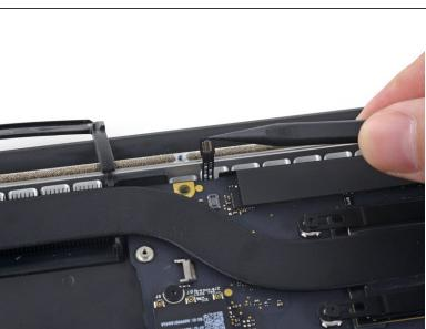
Use the point of a spudger to pry the keyboard backlight connector up from its socket on the logic board.
