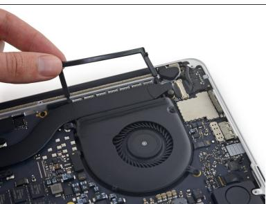
Peel the left rubber cover up off the fan and fold it out of the way.
