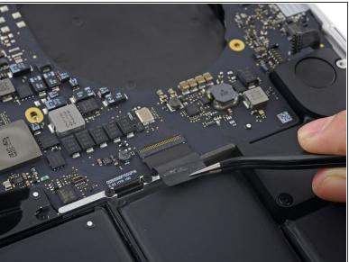
Peel back the tape covering the top of the keyboard data cable connector.
