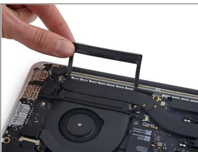
Peel the right rubber cover up off the fan and fold it out of the way.
