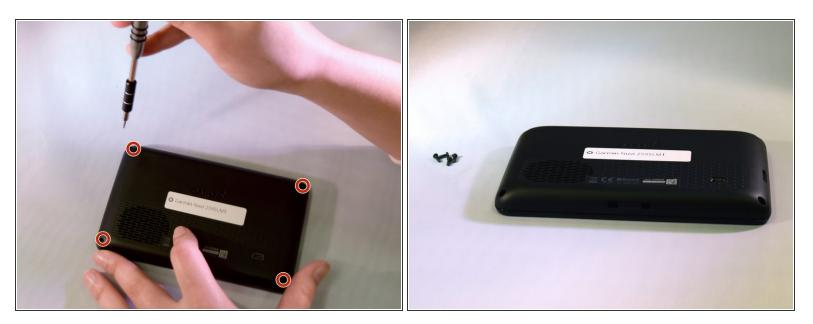
Using the t5 screwdriver from the iFixit Pro Tool Kit, remove all four 5.6mm screws placing them safely on the table.
