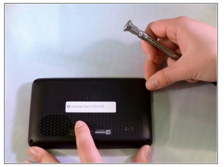
• Place the device on the workspace so the screen is facing downward.
