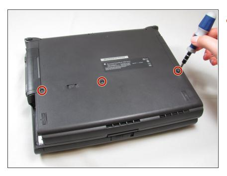
With a Torx T8 screwdriver, remove the three Torx 24mm screws along the center of the back panel.
