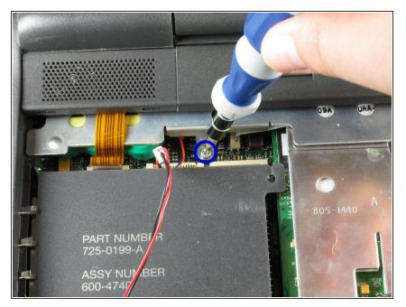
Remove the 7mm screw connecting the speaker panel to the computer.
