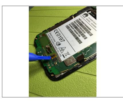
• Unplug the connector that joins the main motherboard with the dock.
