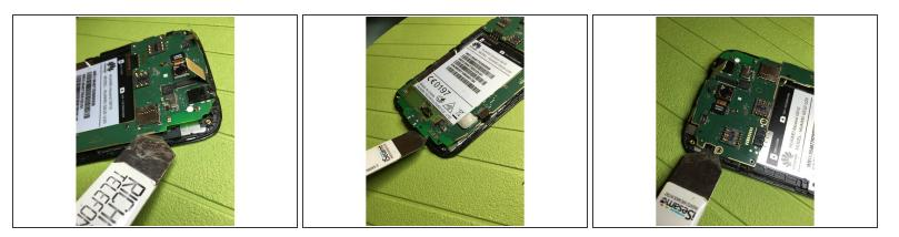
• Unplug the motherboard securely fastened at 3 points and remove it.
