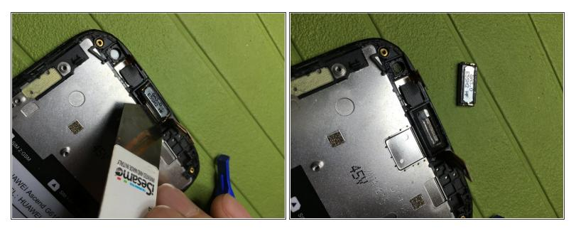
• With the help of a heat source to loosen the adhesive, remove the broken ear speaker and replace it with the new one.
