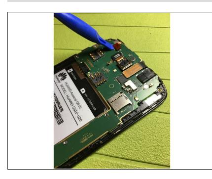
• Remove the ambient light sensor connector.
