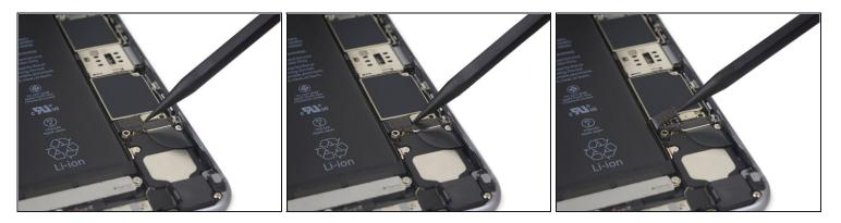
• Use the point of a spudger to disconnect the battery connector by prying it straight up from the logic board.
