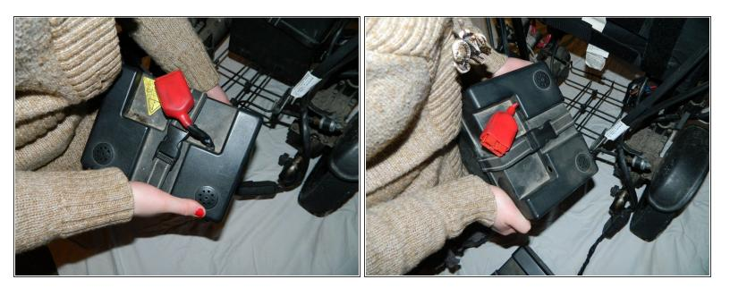
Remove the first and second battery from the wheelchair.
