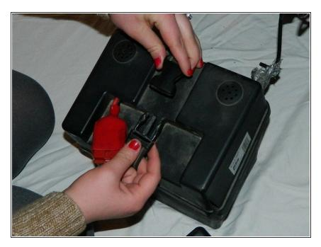
Reattach the clips on each of the battery's protective casings.
