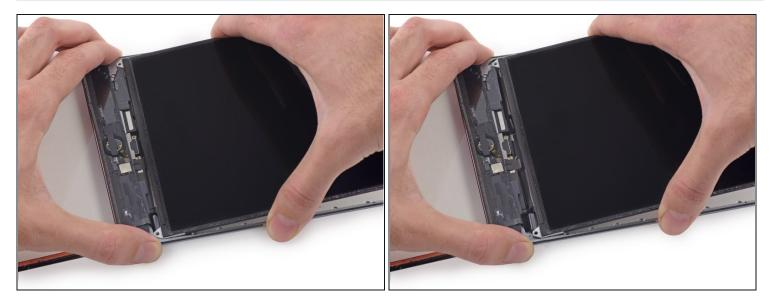
(i) Two wide strips of tape connect the LCD to the speakers.
