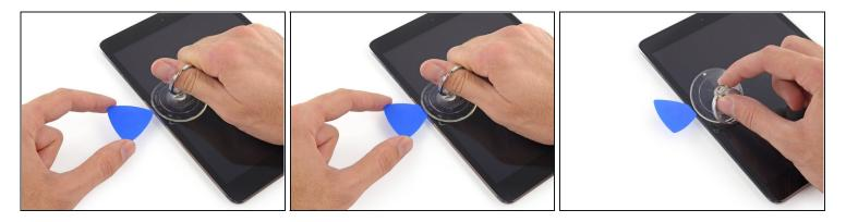
• While holding the glass up with the suction cup, slide the point of an opening pick into the gap between the glass and body of the iPad.
