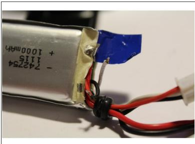
Desolder the two battery tabs with black and white wires connected to them.
