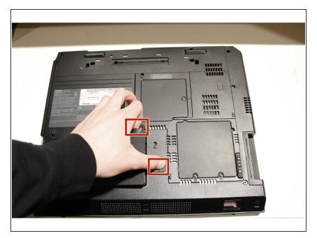
To remove the battery, slide the battery lock lever right, while pulling on the battery tab.
