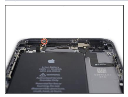
Remove the single 1.3 mm Phillips screw securing the antenna to the rear case.
