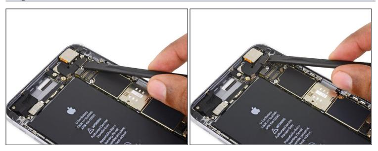
• Disconnect the iSight camera connector from its socket on the logic board.
