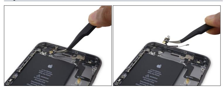
• Remove the Wi-Fi/Bluetooth antenna.
