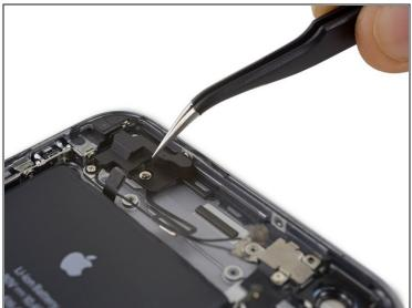
• Remove the sticker over the third screw holding the cellular antenna in place.
