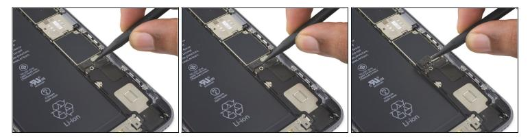
• Use a spudger or a clean fingernail to disconnect the battery connector by prying it straight up off the logic board.
