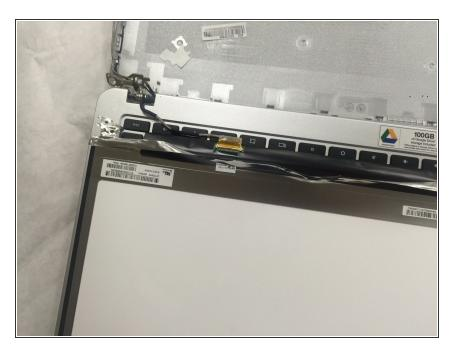
Once you do that, you will see the screen has only one connector. Use the hobby knife to lift up the adhesive tape (Be careful not to cut it) Pull the adhesive tape back, and grab the back of the connector with both your fingers, and gently pull the connector back out. Now the screen is loose.
