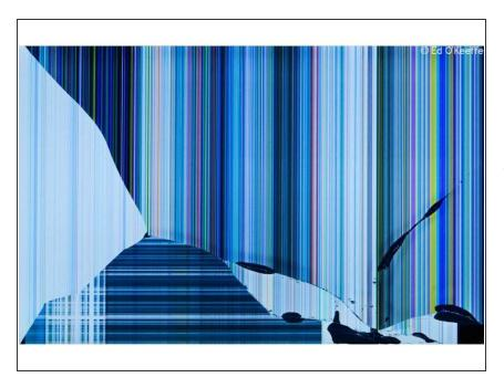
Shattered LED screen is when you push your finger against the screen, you see some kind of a rainbow effect around your finger. If the LED screen is shattered, it is unusable, and needs to be replaced with a new LED screen.
