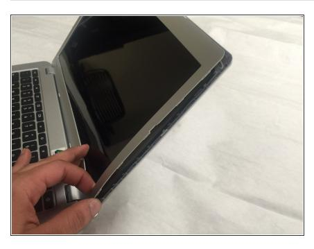
Once you are done with unscrewing, snap off the screen bezel. To do that, you need to reach your fingernails of both hands on the inside of the screen bezel in the left or right side of the screen, and gently lift up and out.
