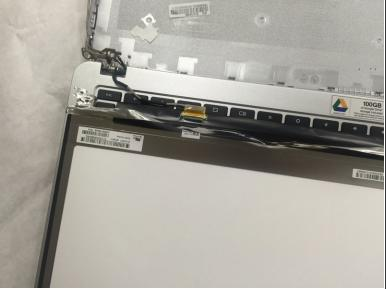
Once you take out the screen bezel, four screws mount the LED screen. Unscrew them, tilt the screen forward, and lay it on the keyboard exposing the backside of the screen.
