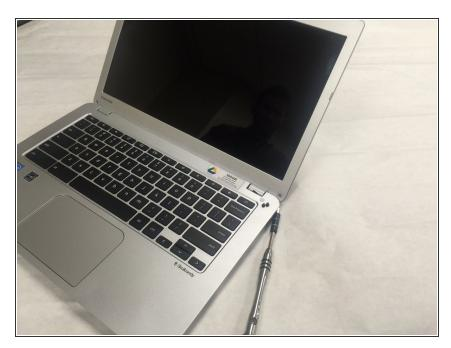
Frist, remove the screw covers with a small hobby knife. Use a PH #0 (Philips screwdriver) to unscrew the couple of screws in the front screen bezel.
