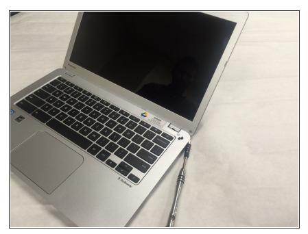
In order to get to the screen assembly, you need to remove the screen bezel (plastic frame around the screen)
