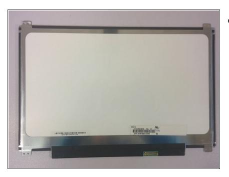
If setting the picture manually did not change the brightness, it simply means that the LED in the back of the LED screen have broke. That means a new LED screen is required.
