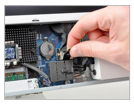
Pull the black plastic tab attached to the display data cable connector to disconnect it from the logic board.
