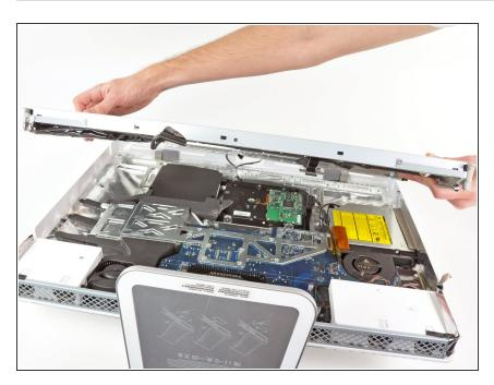
Remove the display assembly from the iMac.
