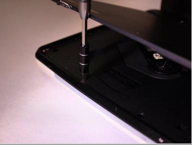
Open the disc flap and remove the screws inside with the Phillips #0 screwdriver. There will be three screws.
