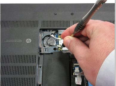
Remove the screw with PH 0 screwdriver that is holding the wireless adapter in. This is PM 2.0x2.5 screws.
