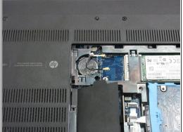
Hold the wireless adapter and gently remove the white and black wires from it. The connectors will come out straight up.
