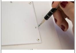
Remove the three 3.5mm screws using the J-0 screwdriver attaching the back panel to the device.
