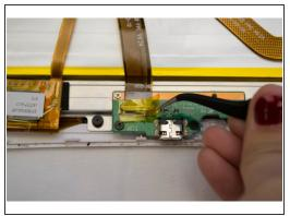
Peel off the yellow tape on the connector from the corner.
