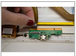
Disengage the white lock keeping the plastic ribbon in place.
