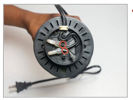
• Lift the two wires from the motor platform.
