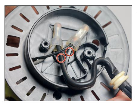
• Using the wire cutters, cut the end of the thick black wires.
