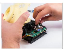
Locate the IR blaster, remove the connecting wire ribbon by prying the connector latch open on the motherboard, then sliding it out. Once the wire ribbon is disconnected, the IR blaster can be lifted away from the motherboard.
