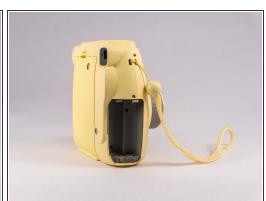
First, push in the lens and remove the two AA batteries.
