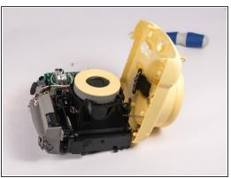
Once all screws are removed, gently pry open the front casing with your hands or plastic opening tools carefully. Do note that there will be a spring that attaches the front casing and the main circuit board, so refrain from allowing excess tension on the spring.
