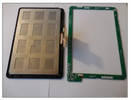
• Separate the screen from the casing and circuit board.
