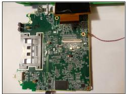
• Lift the motherboard up exposing the fourth and final wire. Once you lift up the motherboard you will need to pull down on the wire to disconnect.
