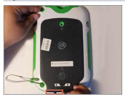
Using a plastic opening tool, pry off the outer protective child proof casing, starting from the bottom.
