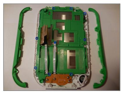
Using the screwdriver with the PH1 bit, unscrew all nine of the exposed screws holding the plastic base down and remove the base.
