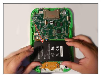
Remove the hard plastic casing, exposing the motherboard and battery.
