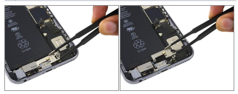
• Remove the Taptic Engine cable bracket.
